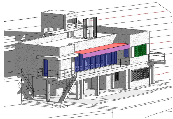
Figure 8. Villa E.1027 winter solstice 12:00. Blue: glass, green: wooden slats, purple: vertical shading, red: horizontal shading.
